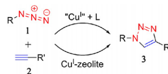
Scheme 1. The Cu I -catalytic systems known to regioselectively promote the Huisgen [3+2]-cycloaddition.
